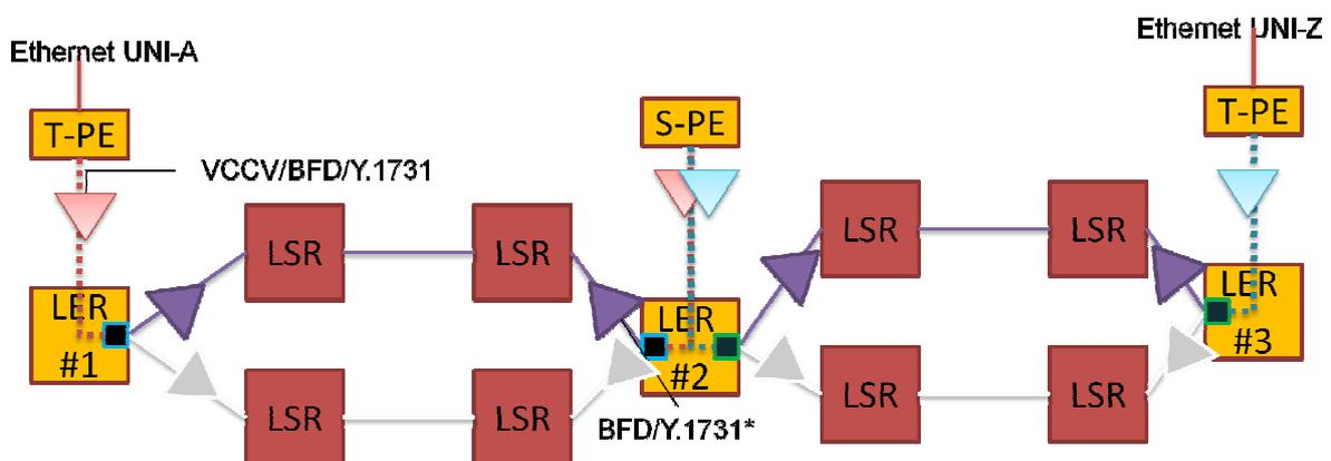
Alarms can be raised on certain events/failures, loopbacks can be used to localize faults and end-to-end connection parameters like throughput, packet loss, latency, latency variation (jitter) can be measured and continually reported. The OAM can be applied across multiple layers across the network. For eg, an End-to-End connection can be monitored, and also for a particular network operator or a particular subnet.
